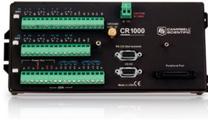
Figure 9.3: Campbell scientific logger using analog communication to receive data signals.
