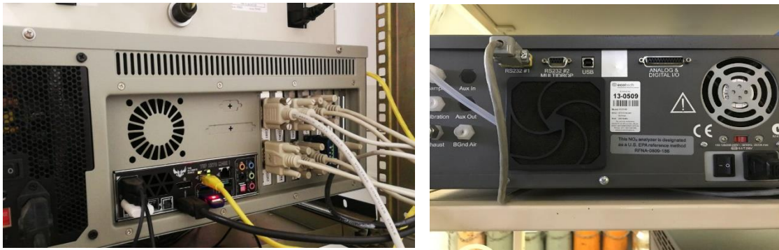
Figure 9.5: Example of serial communication cables used for RS232 communication.
