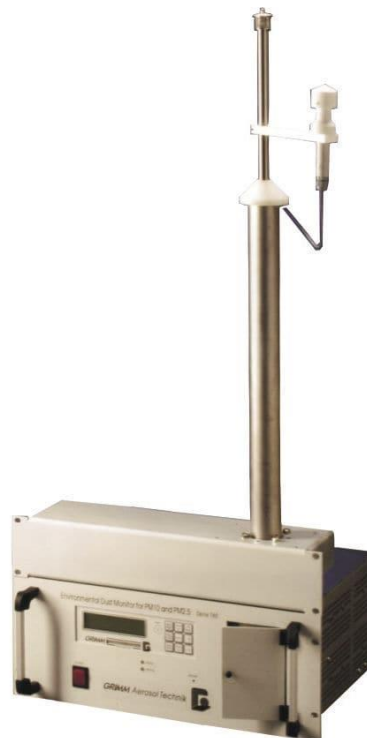
Figure 1.17: PM instrument using the light scattering method
