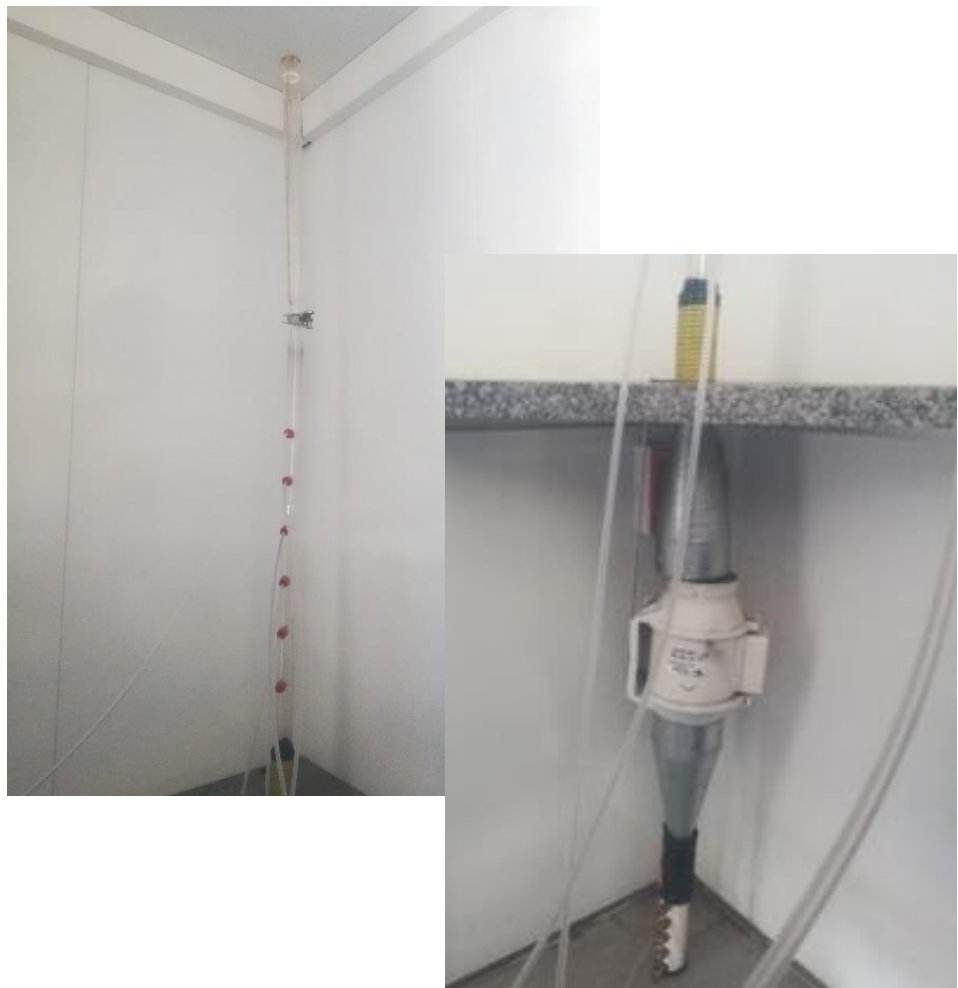
Figure 1.6: Sampling manifold used to draw air into the shelter.
