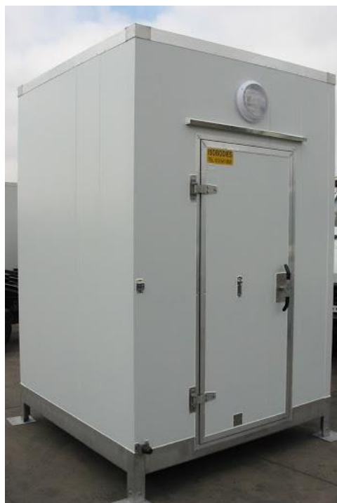
Figure 1.4: Insulated container used to house instrumentation used for measuring air pollution.
