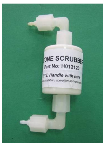
Figure 6.14: Examples of Ozone scrubbers used in an O_3 analyser.
