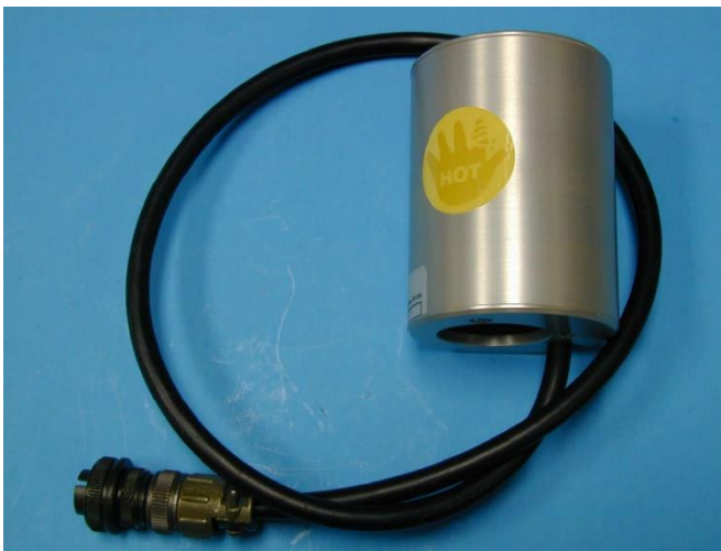
Figure 8.8: Inlet sample heater.
