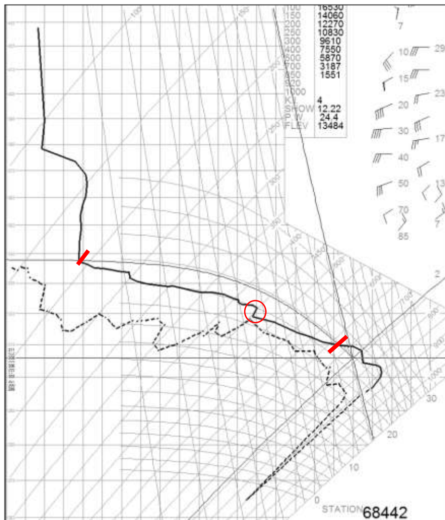
Figure 31: Tephigram for Bloemfontein indicating Normand's theorem calculation for the cloud base (thick red line) and cloud top height (thick red line) for the convective clouds at 00h00Z (SAWS, 2007).
